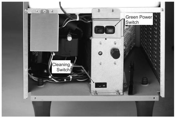
Front View With Front Panel Removed
